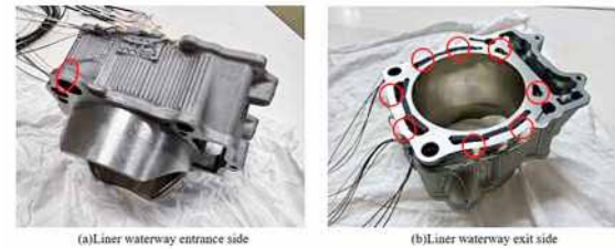
Fig.3 Cylinder Block with thermocouple
