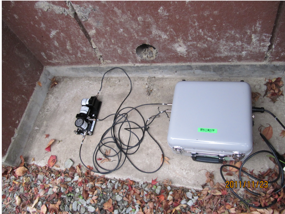
(a) Measurement with the sensors in three components and data logger A
