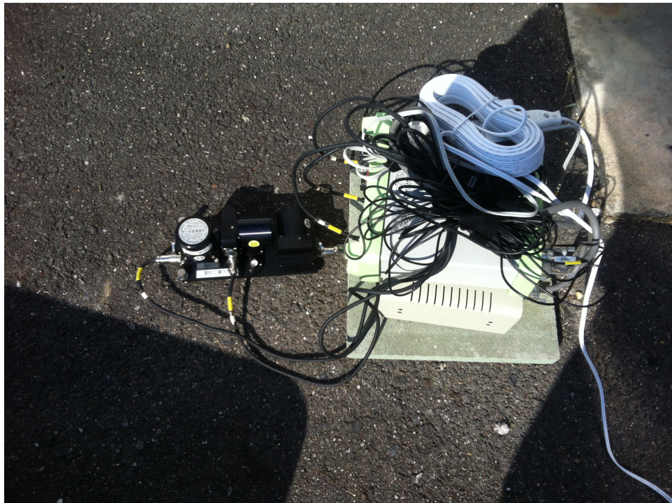
(b) Measurement with the sensors in three components and data logger B
